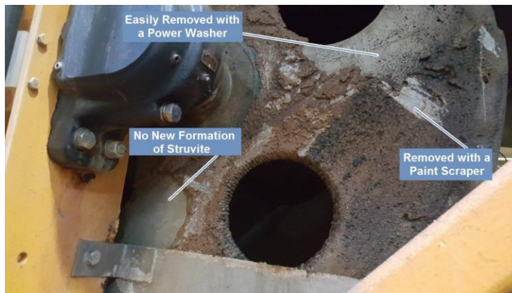
Figure 6: Condition of BFP Drum Surface at the End of 90-day Test Period
