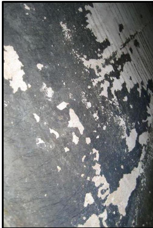
After 150 days of *HydroFLOW* operation - 1mm of brittle scale remains
