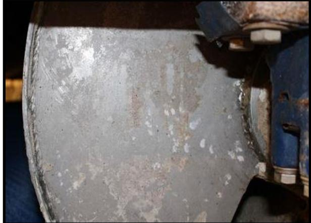
After 150 days of *HydroFLOW* operation - Very little scale, no chemical or mechanical scale removal performed
