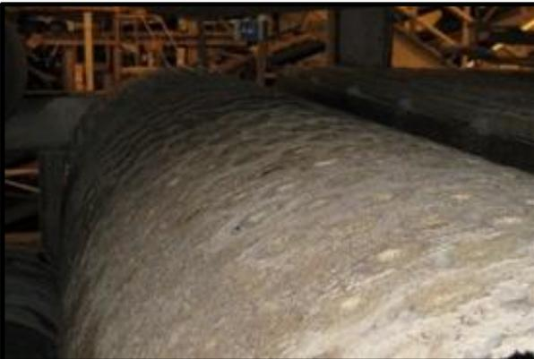
Before - Hard scale and bridged-over holes
