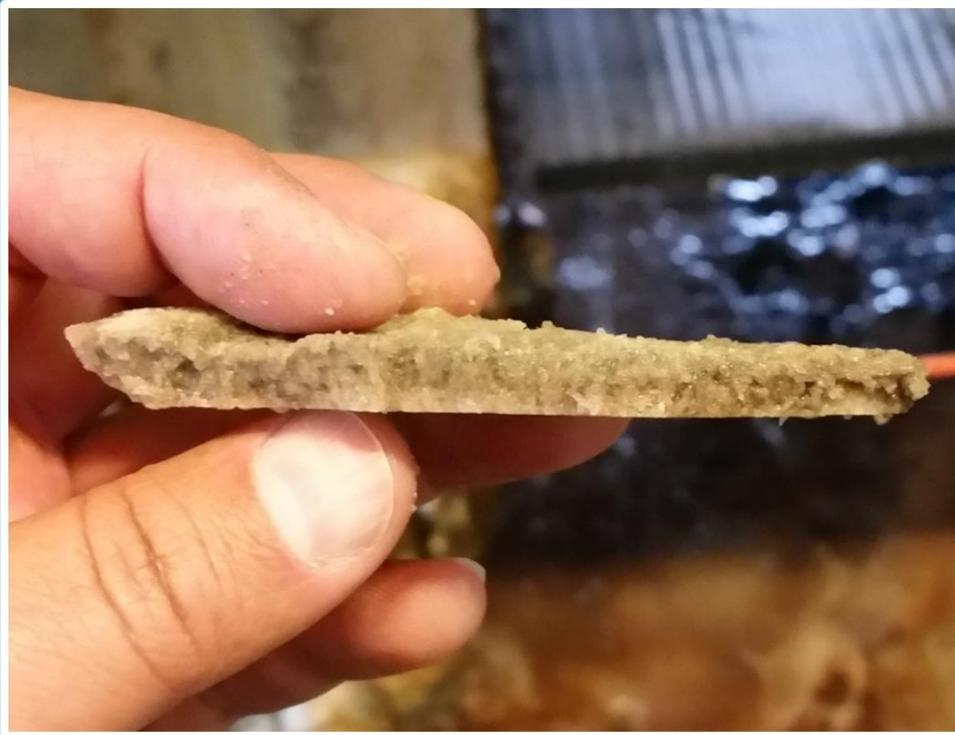
1/4 INCH STRUVITE BUILD-UP INSIDE THE BELT PRESS
