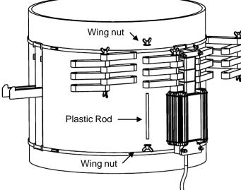
Adjust position of ferrite support brackets if necessary
